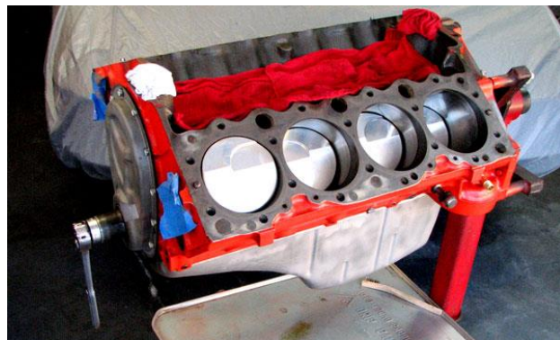
Engine being readied for assembly. Cylinder heads are still out for rebuild.
