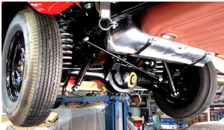
Inspection war paint (yellow circle) identifies rear end gear as Positraction during assembly process.
