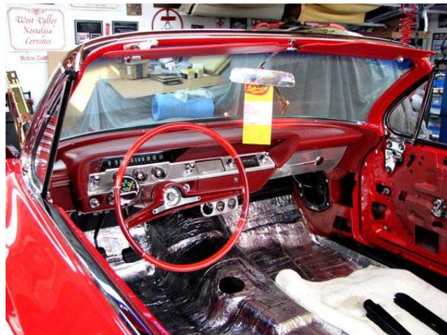
Interior is freshened up original along with the dash pad. No Repro Here! Dynamax blankets are added to body floor to make riders more comfortable as dual mufflers are located under the floor.
