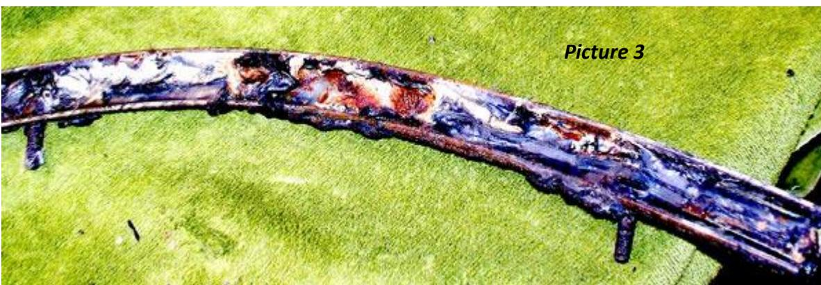
We cleaned the frame with solvent, plastic chisels, and paint thinners. Once the parts were clean, we were surprised to see that the metal work was in very good condition. There was only surface rust on the lower window channel, which we removed with phosphoric acid picture 4 on the next page.
