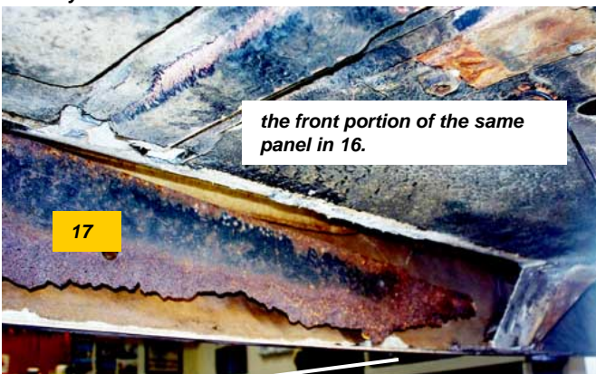
Metal remaining after removing Inner Rocker Panel
