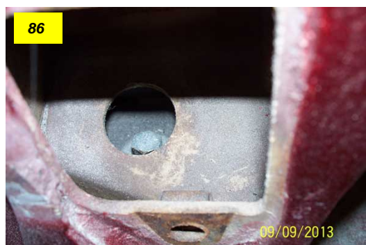
View from above of the rear bolt in the pillar support. This is looking through the area where the door hinge would fit.
