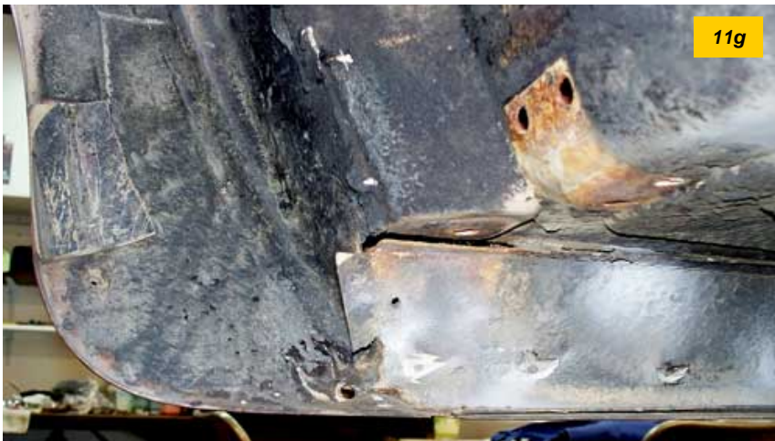
(ABOVE) a view of the rear of the fiberglass panel below the rocker that was to be removed to allow us to see the metalwork. It is partially pried away from the body.
