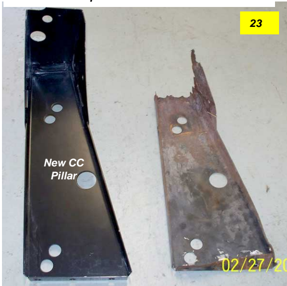
(Below) A comparison of the old and new pillar supports, once the old one was removed from inside the kick panel.
