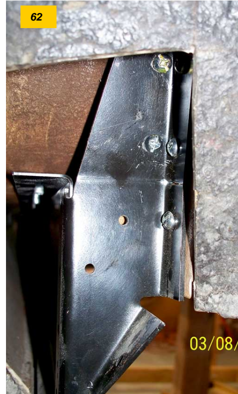
(BELOW) A view from the rear showing the bolts going through the inner rocker panel support, through the fiberglass, and into the new rear body mount reinforcement.
