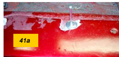
rear view of the new inner rocker panel support in place, ready to be riveted in place.
