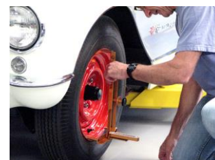
Joe prepares to measure the Airbox Caster & Camber.
