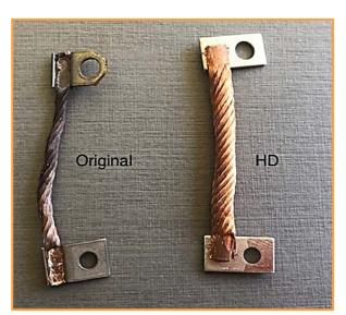
Left, the original lead is burning. Right, the heavyduty replacement. The leads are found here #4 in the starter diagram below.
