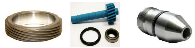
OEM AC Delco gears were used in Muncie, GM T10, GM Super T10, Saginaw 3 & 4 speed, GM T5, Powerglide, and 200 & 350 transmissions. We are going to concern ourselves with the Muncie, T-10, Saginaw 3 speed, and Powerglide here. There are various gear sizes and number of teeth that will produce different speedometer readings. First we are going to discuss what might be used in the transmission.
