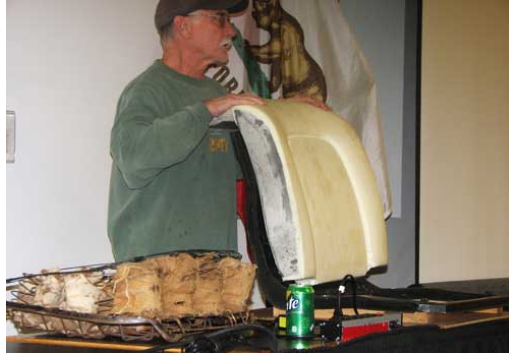
Molded seat back cushion on frame.
