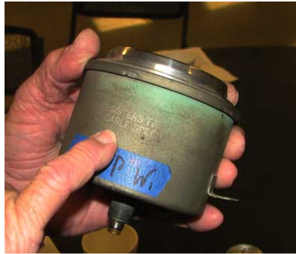
Stamped usage lettering on Tachometer Case.
