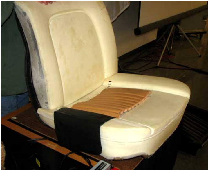
Newly fabricated foam supported back and bottom seat cushion. Also ribbed material for added comfort.
