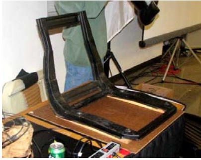
Basic seat frame on a '60 C1.
