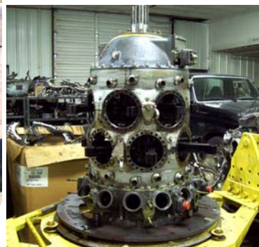
One of our engines being overhauled to new condition (Pratt & Whitney R2800, 18cylinder, 2000hp).
