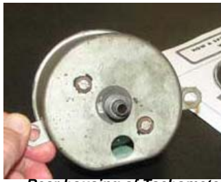
Rear housing of Tachometer with instrument light hole.
