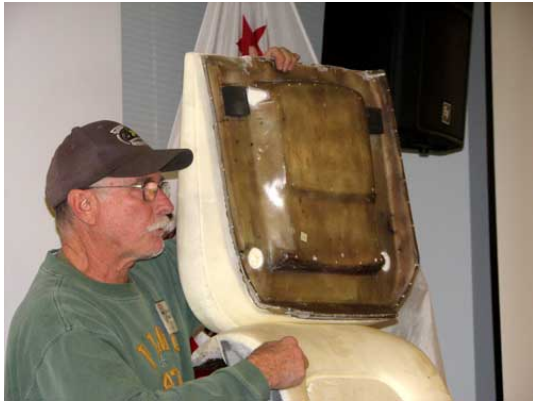
John's fiberglass molded seat cushion with more stronger side support and foam base. Assembly sits into original frame.
