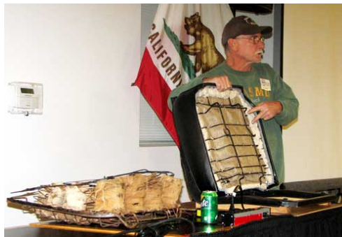
A properly rebuilt seat cushion with restrung springs.
