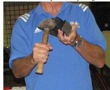
Brake Shoe fit to Brake Drum should be checked and adjusted. Hammer technique shown below works. Secure shoe in vise prior to adjusting.
