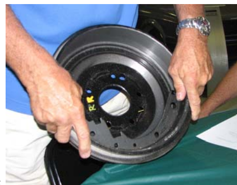
Brake Shoe fit to Brake Drum should be checked and adjusted. Hammer technique shown below works. Secure shoe in vise prior to adjusting.
