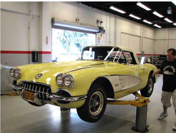
Prior to lifting, Chip checks to verify Emergency Brake is off, Transmission is in neutral and he is about to raise the hood.
