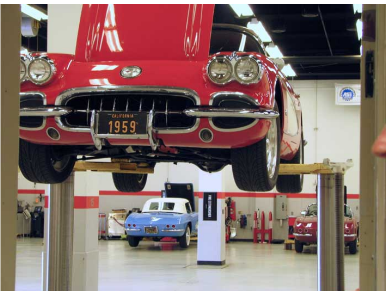
Prior to lifting, Chip checks to verify Emergency Brake is off, Transmission is in neutral and he is about to raise the hood.
