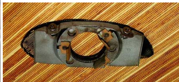
(Top & Bottom) Special clamp for '57 - '60 Vettes where exhaust extends through rear bumper.
