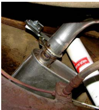
Exhaust pipes "snaking" through the center X-member.
