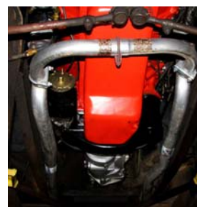
Cross over pipe is used on Large HP Engines
