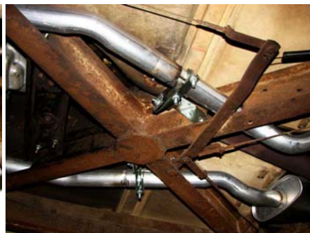
Exhaust pipes "snaking" through the center X-member.
