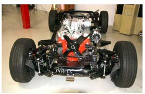
Pictured at the left is Kent's current project, an "air box" '57 racing Corvette. The chassis is in the final stages of completion featuring a 283" FI engine, big brakes, large fuel tank, and on and on. The body is currently being completed and detailed. The body color will be white as indicated by the "white" war paint painted on the front chassis cross-member.
