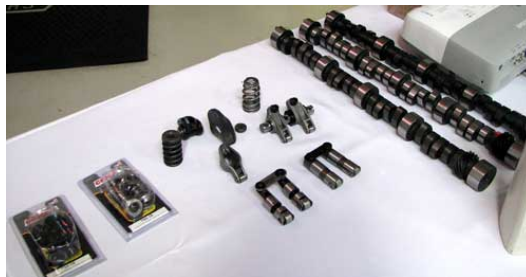
(left) Engine hardware includes flat & roller tappet, roller rocker arms and flat & roller cams
