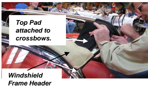
Top frame assembly with windshield and deck frame members remaining along with the Hinges.
