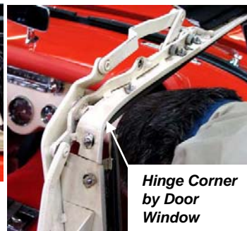
Top frame assembly with windshield and deck frame members remaining along with the Hinges.
