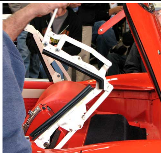
Folding sequence for the side hinge assembly on the '56 - '62 Convertible Top Frame.
