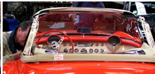
Top frame assembly with windshield and deck frame members remaining along with the Hinges.
