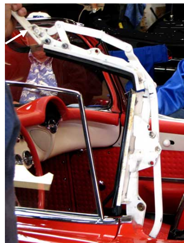
Front folding hinge piece to interface windshield header.
