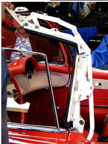
Folding sequence for the side hinge assembly on the '56 - '62 Convertible Top Frame.
