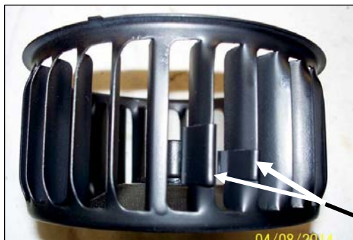
Picture 16-1: Fan Blade Balance Weights
