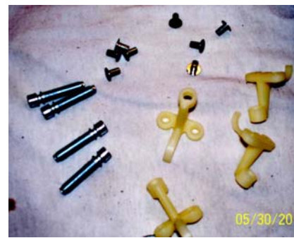
Picture 25: CC kit for headlight bucket repair.
