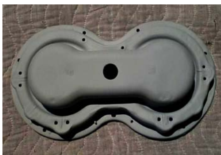
Picture 23: Primer coated headlight bucket.
