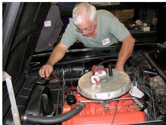
Coolant level and Coolant electrical conductivity is checked by Joe Fekete.
