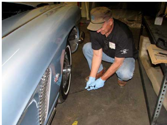
Steve Clifford checking looseness in front suspension.
