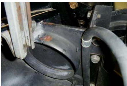
Picture 10: Hood support interferes with air duct entrance.
