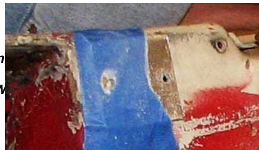
Taped on sheet metal covering existing old screw hole. 1/8 inch holes to the side are drilled through door and will house the pop-rivets.
