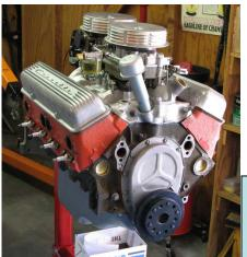
Original block, 30 over 292 ci. Ported cylinder heads, hydraulic roller cam with original dual quads. Dyno results 304hp at 6000 rpm. Torque 314lbs @3700rpm. Note that factory specs were 283ci, 245hp @5000, and 300lbs torque @3800rpm.
