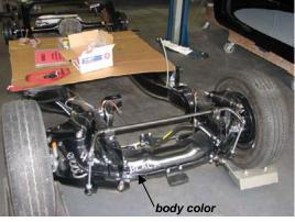
The front crossmember on the chassis contains the code indicating the body color that will be assembled down the line. This "written" color provides a cross check to the assembly person that a black body will be set on the frame. If the color written does not match the body color, everything stops.
