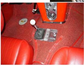
4. The overall fit of the transmission into the car is tight. (There is less than ½" clearance between the top of the transmission and the fiberglass tunnel in my 1960. I have not seen any evidence of the transmission hitting the fiberglass after 5000 miles. I assume that it is also OK for the 1958 and 1959 models because of body style similarity. I do know that there is a major clearance fit problem with the 1957 model. (See member John Costales for details)
