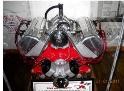
(Above) Duntov 1947 engine (flat head) with Duntov OHV conversion.
