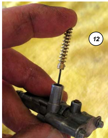
Photo 12) Insert the core wire back into the sheath and housing.
