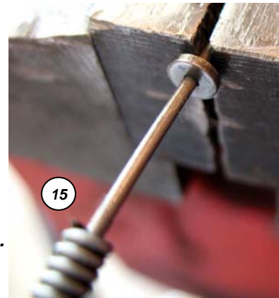
Photo 13) Measure the working end of the wire about 1/8" longer than your original reference measurement.
