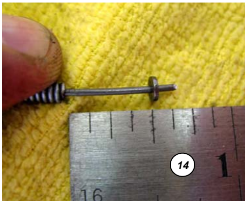
Photo 14) Replace the washer "stop" to the correct length.
