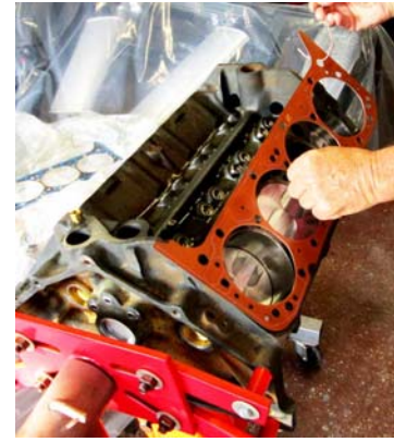
Cylinder Head Gasket placed on Engine Block.
