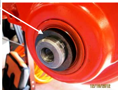
Vibration Damper spacer on crankshaft.
