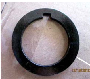
Vibration Damper spacer on crankshaft.
