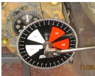
Engine rebuilder visit to check cam degree with his equipment.
