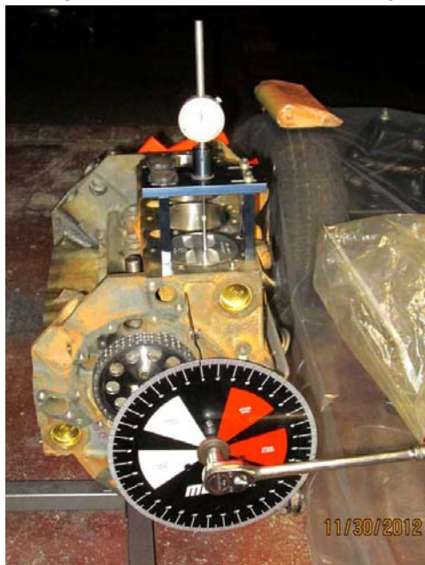
Engine rebuilder visit to check cam degree with his equipment.
