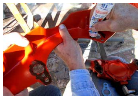
Gasket Seal applied to both sides of Engine Mount.
