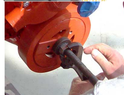
Vibration Damper Install using special tool (used by Steve Clifford)
