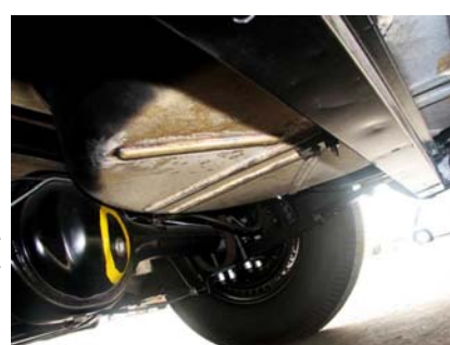
Right) View under rear of '57 shows sample of War Paint applied by factory indicating which rear differential was installed per the original customer order.
