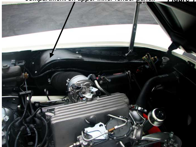
"Air Box" located on left side of engine compartment on upper inner fender panel. Figure 1
