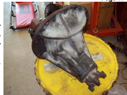
Typical Chevy rear-end center section, referred to as the "pumpkin".
