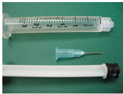
Photo 3: You need a 3cc syringe with a micro tip (.025") which you can obtain at a hobby shop or from any of the many SACC members who are dentists.
