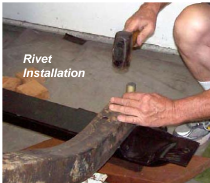
(left) Rivet installation to attach new cross-member. (top) Frame surface prep for welding (right) new battery tray.
