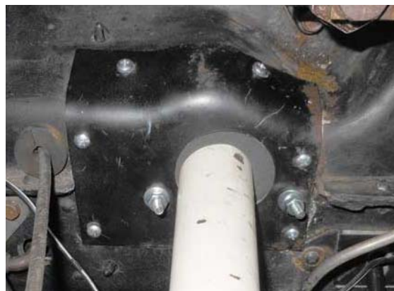
New split Inner Grommet with pop rivets and aluminum plate.
