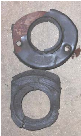
Upper picture of hard inner grommet with rubber and metal inside. Lower soft inner grommet.
