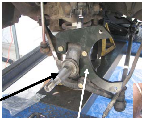
Caliper Mounting Plate bolts to original backing plate bolt holes.
