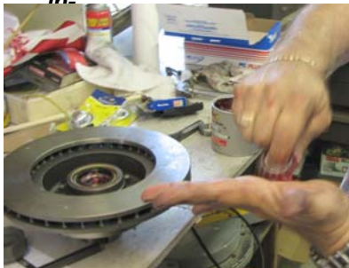
New Disc/Hub assembly requires inner and outer bearing races to be removed and replaced. All parts are supplied.
