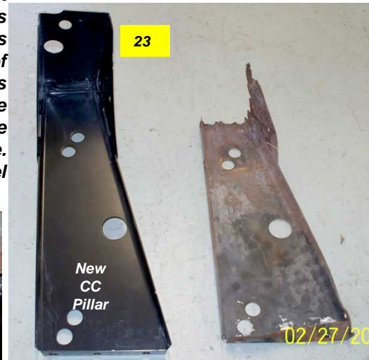
(ABOVE) A comparison of the old and new pillar supports, once the old one was removed from inside the kick panel.
