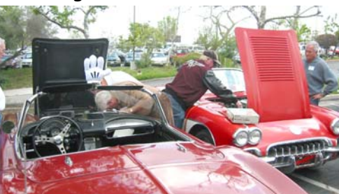
(left) Neil Fraser's '58 gets a hot shot to try and overcome a bad solenoid. A subsequent "push start" worked.
