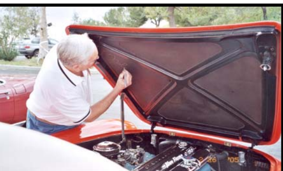
(left) Neil Fraser's '58 gets a hot shot to try and overcome a bad solenoid. A subsequent "push start" worked.
