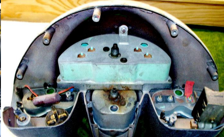
Picture 9 is a view of the rear of the gauge cluster intact. Picture 10 shows the oil gauge and the ammeter, with a radio static suppressor capacitor attached.
